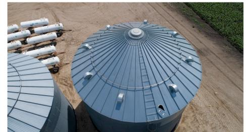
**BIN 5:** 35,000± bu. Butler bin, Y design floor aeration, side ladder, Edwards grain guard IL24-5-1, 5 hp. Squirrel 230V 30 amp single phase cage fan, Rapat bin system powerhead loadout auger, 7.5 hp. Blador motor, electrical panel w/(1) 110V & (2) 240V outlets
