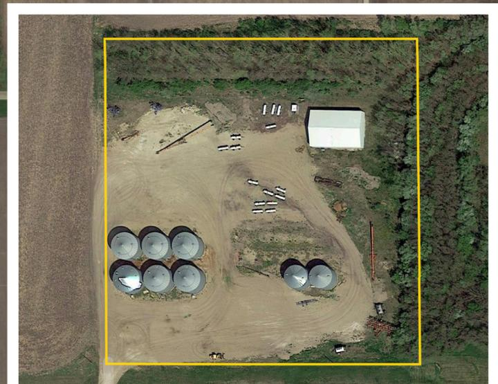
**BIN 1:** 35,000± bu. Butler bin, Y design floor aeration, ladder, Butler 443985 230V 42 amp single phase fan, Rapat bin system powerhead loadout auger, 5 hp. Baldor motor, electrical panel w/(1) 110V & (2) 240V outlets, damage to west side
